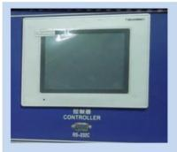
Programmable LCD controller, can do cyclic test with temp, humid, water spray and condensation.
